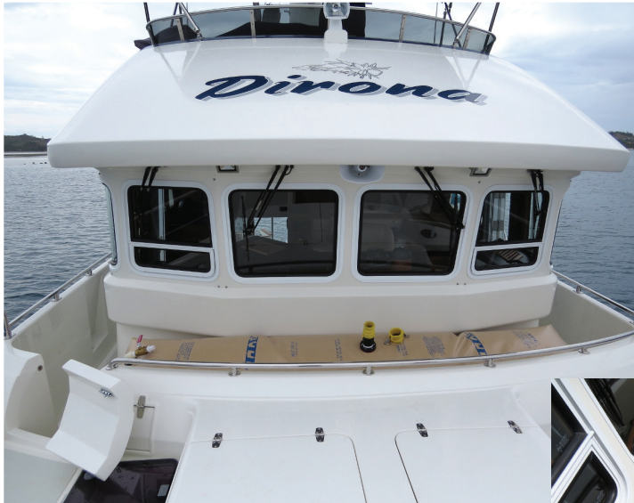
James and Jennifer Hamilton on the Nordhavn 52 Dirona used a 360-gallon ATL bladder designed to fit into their Portuguese bridge, left and below.
