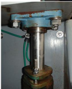
Above, rudder post with tiller attached to steering ram. Note padded rudder stops and two autopilot sensors. Left, rudder bearing mounted above, rudder tube coupling below.
