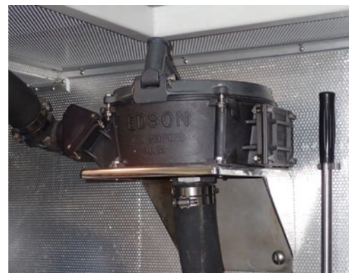
Left, the classic hand-held pump comes in handy when bailing out a dinghy. Above, a high-capacity Edson diaphragm pump with its handle stored nearby.
