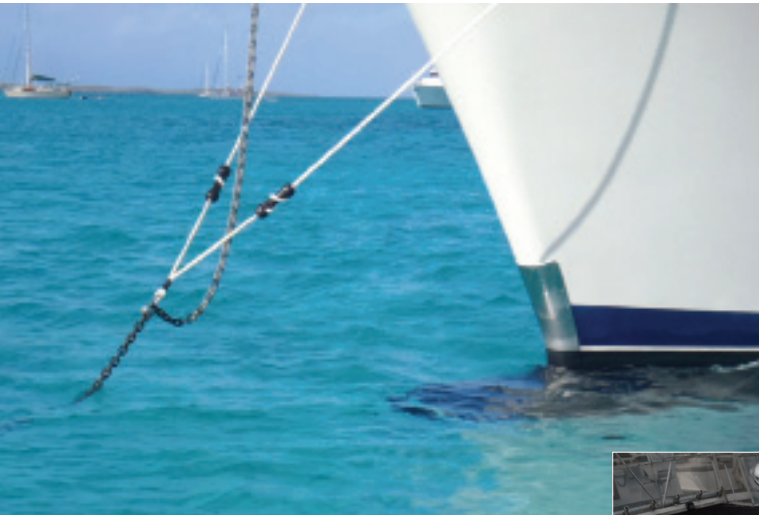
Above, an anchor bridle setup evenly distributes the load. Right, an anchor keeper made from StarBoard keeps the anchor firmly in place.
