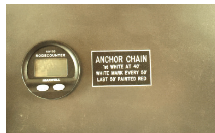
Marking your chain at various lengths lets you know how much you’ve deployed. Above is a plate in the pilothouse that reminds crewmembers of the code.
