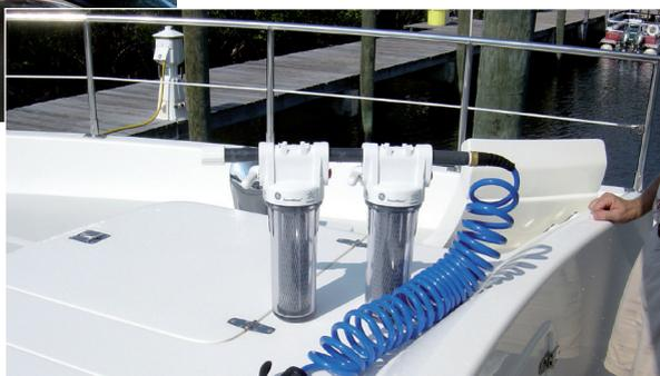
Above, a Seagull IV water purifier tap. Right, a dual-filter system for cleaning dock water.
