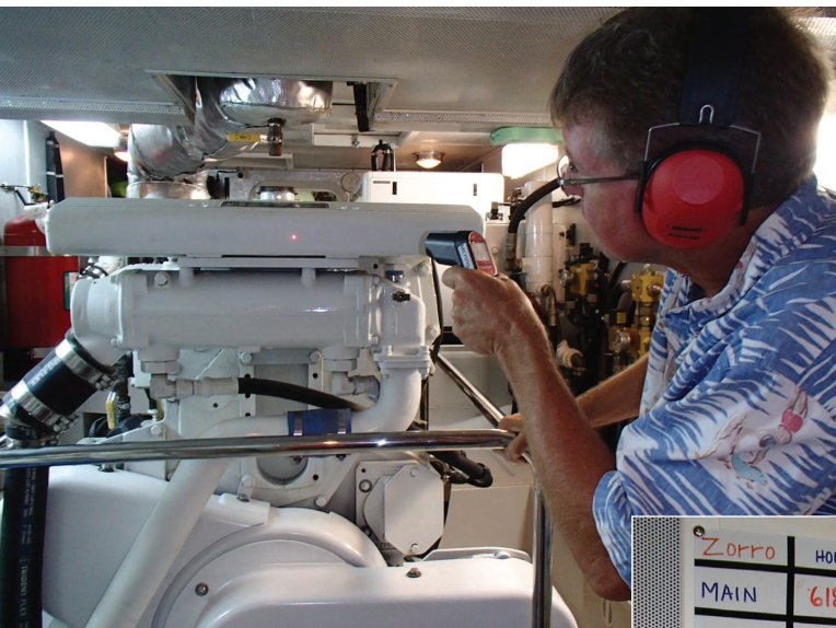
Left, the author doing an engine room check with infrared thermometer gun (note ear muffs for sound protection). Below, dry erase boards are a simple way to keep track of engine room maintenance.
