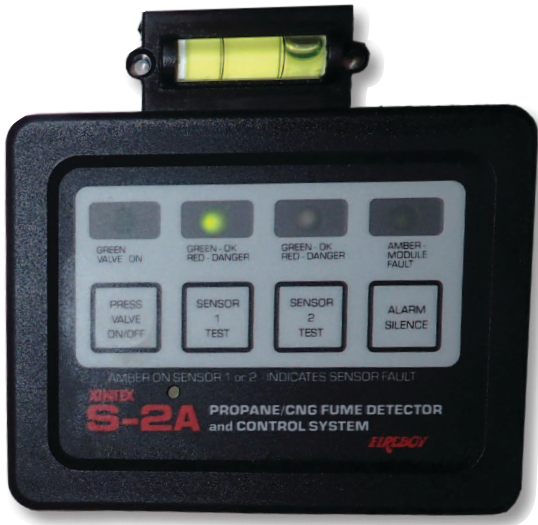
Above, a propane alarm unit. Right, a fire suppression status panel for monitoring the engine room.
