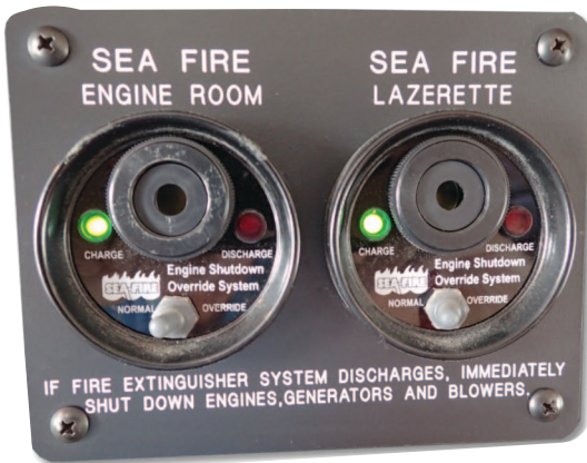
Above, a propane alarm unit. Right, a fire suppression status panel for monitoring the engine room.
