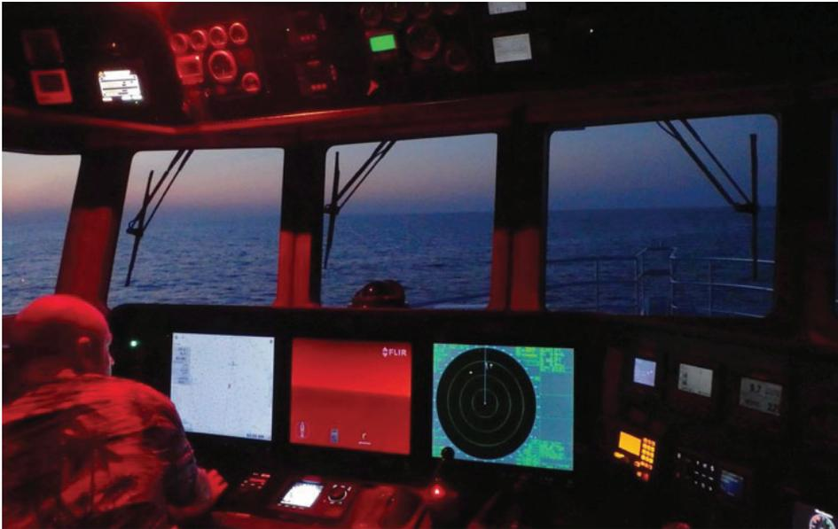
Above, a modern pilothouse with multiple screens can put out considerable light. Dimming the screens helps preserve your night vision. Right, a tidy instrument cluster on a Selene 59.
