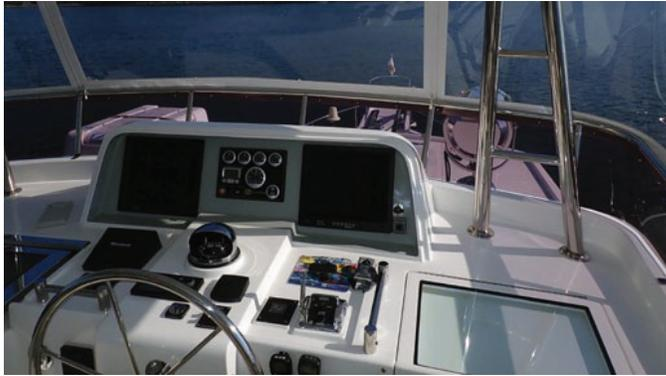
Most flybridges have a duplicate set of instruments and controls.
