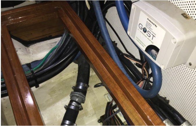
Left, a Global Ocean Security Technologies bilge pump monitor unit.
