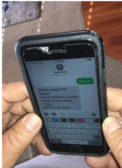
Above right, an iSocket shore power monitor unit plugged into a boat's AC outlet. Right, a smartphone text from the iSocket reporting on system status.
