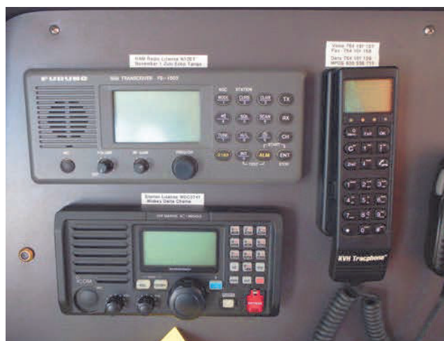
Left, labeling helps. Here are an SSB, a VHF and a satphone all labeled with info for easy operation. Below, a VHF with an emergency procedures checklist.
