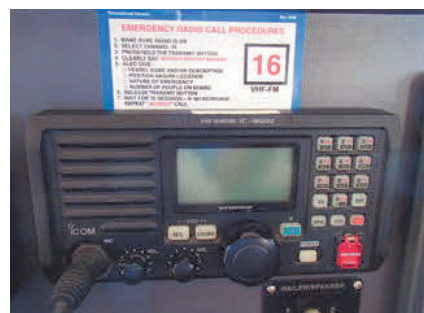
Left, labeling helps. Here are an SSB, a VHF and a satphone all labeled with info for easy operation. Below, a VHF with an emergency procedures checklist.
