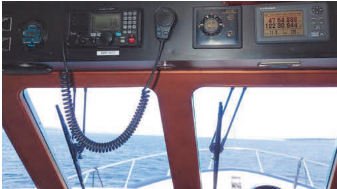
A VHF in the pilothouse with a dangling mic cord. This can be kept out of the way with a simple coat hook.
