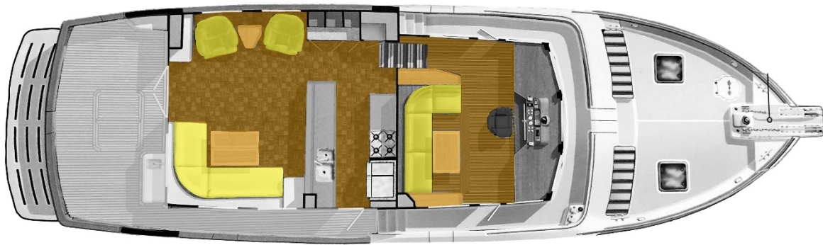
Layout: Lower-level engine room aft, with staterooms and heads forward
