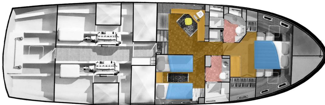
Layout: Lower-level engine room aft, with staterooms and heads forward
