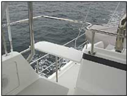
To add another "perch" in the flybridge, P.A.E. added a bench seat welded onto a custom stainless railing.
